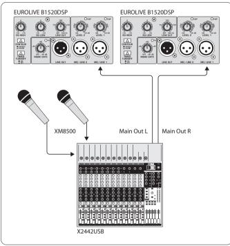
Fig. 4.2: Connecting a mixing console
